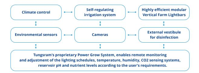
The fully automated system sends an alarm to users via e-mail when any of the parameters are out of range and supports data collection for offline analysis.
